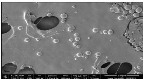
Fig 7. SEM of selected microspunge (Magnification x500)
