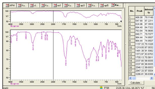
**Fig 3. FTIR of drug & polymeric mixture**
