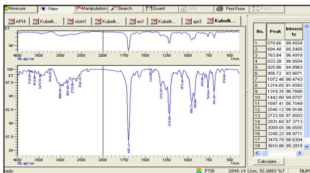
**Fig 2. FTIR of Flurbiprofen**
