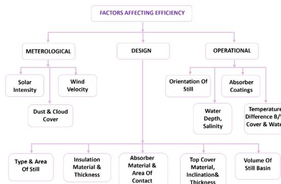
Figure 4: Various factors effecting efficiency of Solar Still.
