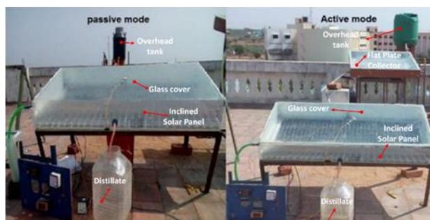
Figure 3: Experimental configurations of the inclined solar panel basin still [3].
