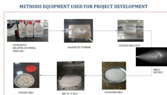
Figure 2. Sequential rotating-pan spray-coating process for the preparation of biopolymer-coated urea granules
