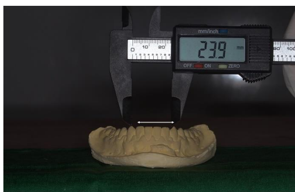
[Figure 2] Measurement of intercanine distance in mandibular arch using digital vernier calliper
