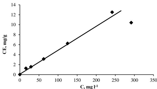
Figure 4. Adsorption isotherm of Cerium with the PANI / CNT nanocomposite.
