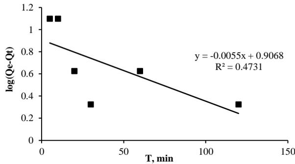
**Figure 6.** Linearization of kinetic data on cerium adsorption on a PANI / CNT nanocomposite using a pseudo first-order model.
