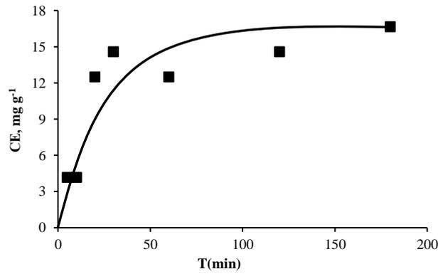
**Figure 5.** Integral kinetic curve of sorption of cerium on a nanocomposite - PANI / CNT
