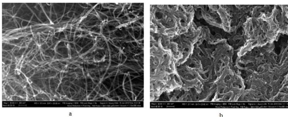
**Figure 1.** SEM images of the initial CNT “Taunit-M” (a) and the PANI/CNT (b) nanocomposite.
