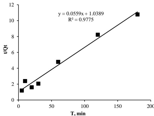
**Figure 7.** Linearization of kinetic data on cerium adsorption on a PANI / CNT nanocomposite using a pseudo-second order model.
