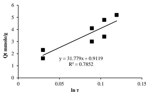
**Figure 8.** Linearization of kinetic data on the adsorption of cerium on the PANI / CNT nanocomposite according to the Elovich model. Kinetic constants obtained by processing data on pseudo first and pseudo second order models and the Elovich model [23] (Table 1) indicate that the kinetics of cerium adsorption on the PANI/CNT nanocomposite with a higher correlation coefficient is described using a pseudo second order model.
