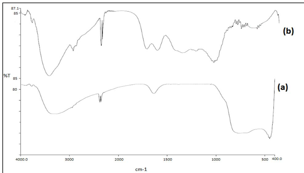
**Figure 2.** FTIR spectra of (a) TiO<sub>2</sub> NPs synthesized by sol-gel method, and (b) pomegranate peel
