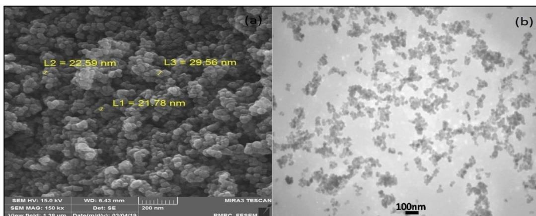
Figure 3. a) SEM and b) TEM images of TiO<sub>2</sub> NPs synthesized by sol-gel method
