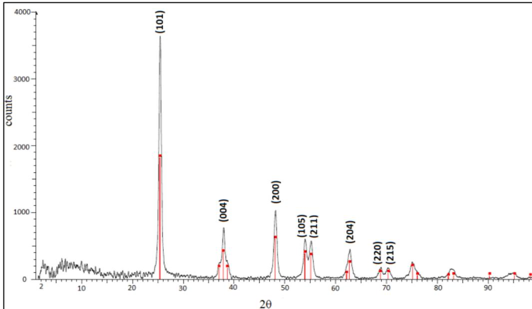
**Figure 1.** XRD pattern of TiO<sub>2</sub> nanoparticles synthesized by sol-gel method
