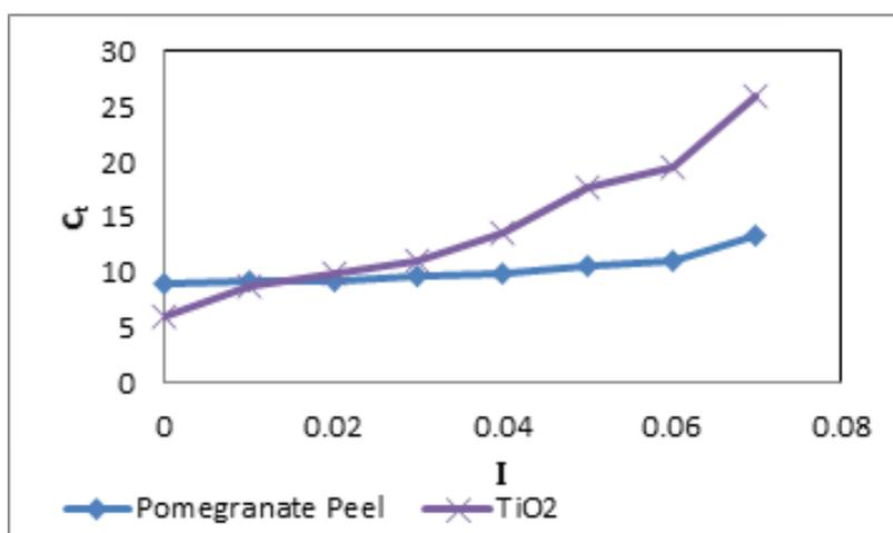
Figure 4. The effect of ionic strength on the Ni<sup>2+</sup> adsorption by TiO<sub>2</sub> NPs and pomegranate peel
