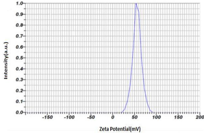
Figure 6. Surface charge of TiO<sub>2</sub> nanoparticles measured by zeta potential.
