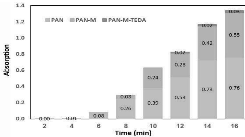
Figure 4. The variation of absorption of HCN from solution as a function of time for different nanofibrous filter media.
