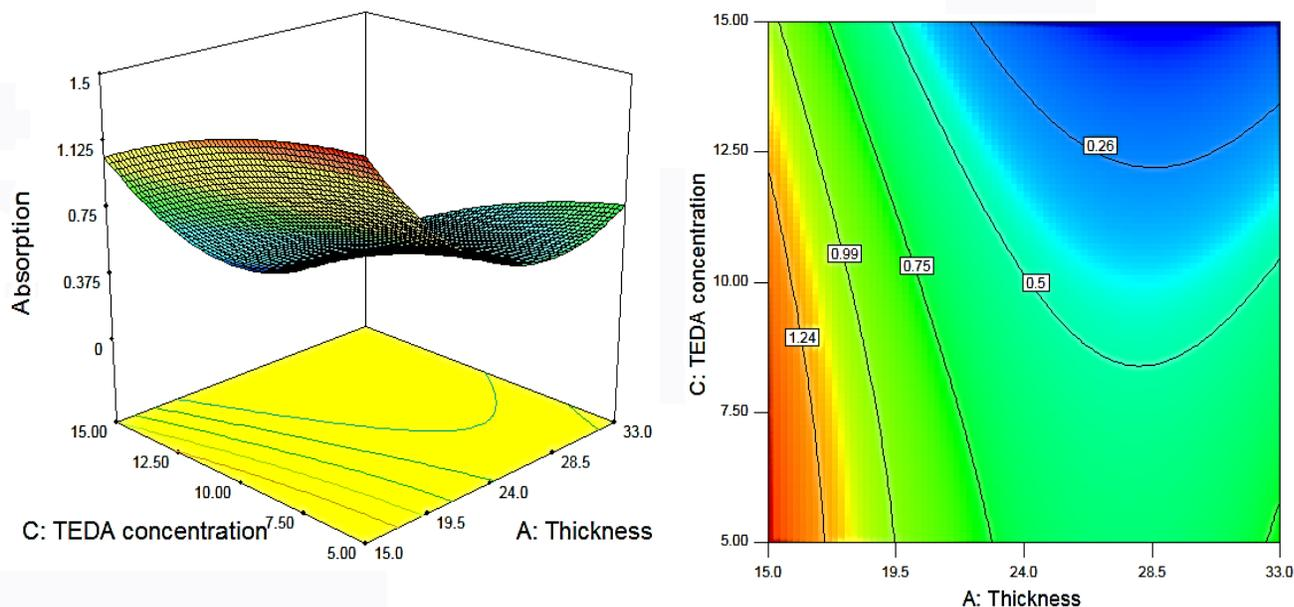
Figure 7. Response surface and contour plot for absorption of HCN from solution.
