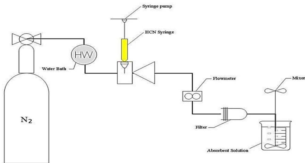
Figure 1. Schematic representation of filtration process.
