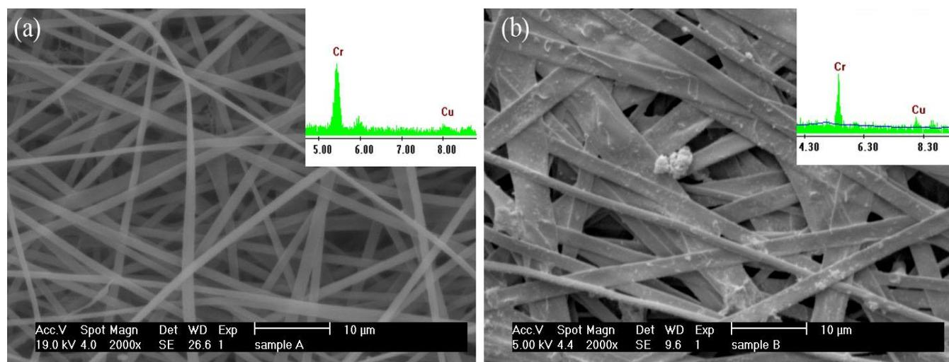
Figure 2. SEM images and EDX spectra of (a) PAN-M and (b) PAN-M-TEDA nanofibers.
