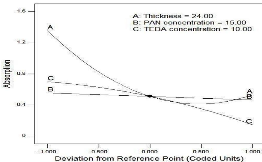
Figure 6. Perturbation curve for the absorption of HCN from solution.
