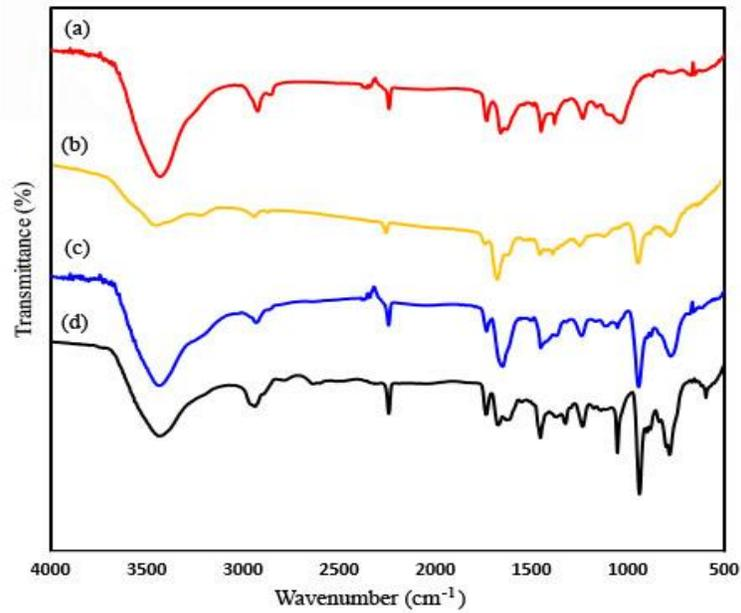
Figure 3. FTIR spectra of (a) PAN, (b) PAN-M, (c) PAN-M-TEDA and (d) PAN-M-TEDA-HCN nanofibers.
