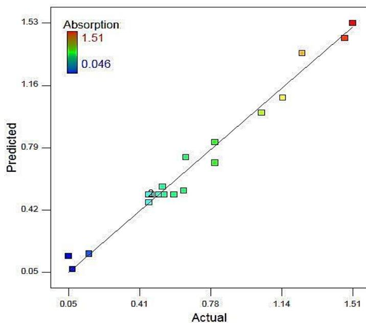
Figure 5. Comparison between the actual and predicted value of HCN absorption from solution.
