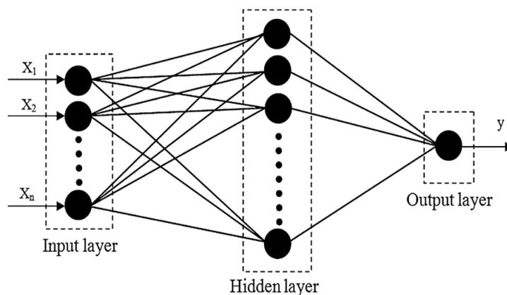
**Figure 1.** A three-layer MLP neural network model
